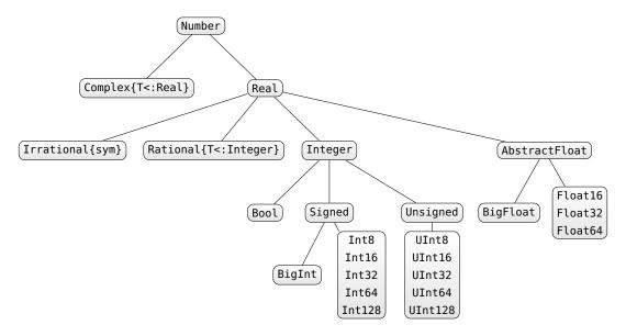
Figure 1: Hierarchy of numeric types
